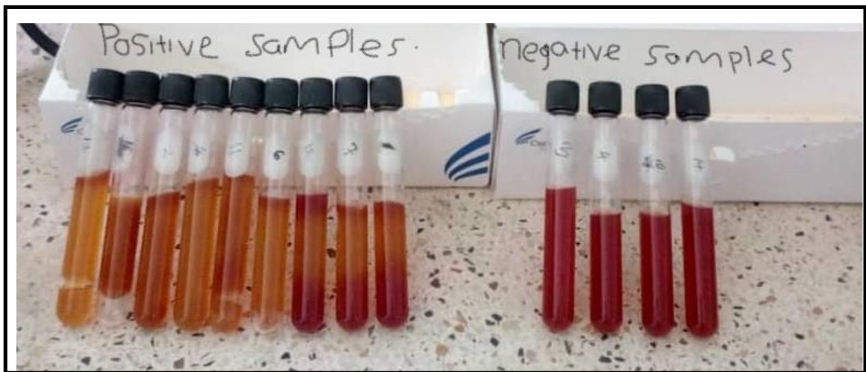
Figure 23: Positive and negative samples for total coliforms / E. coli presence in test tubes
