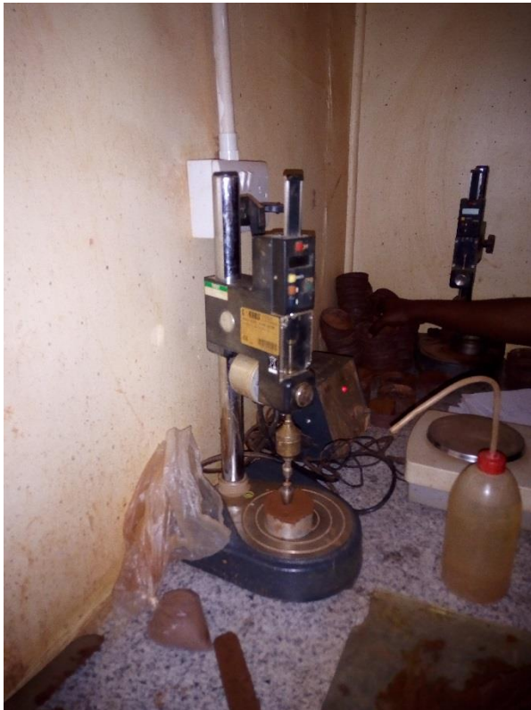
Figure 5: sample penetration by the penetrometer
