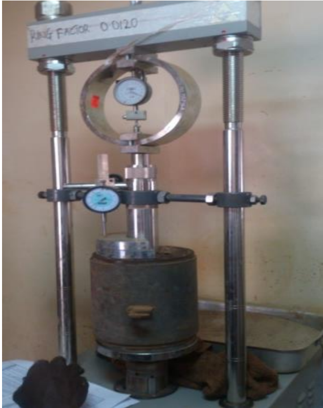
Figure 10: CBR testing machine.
