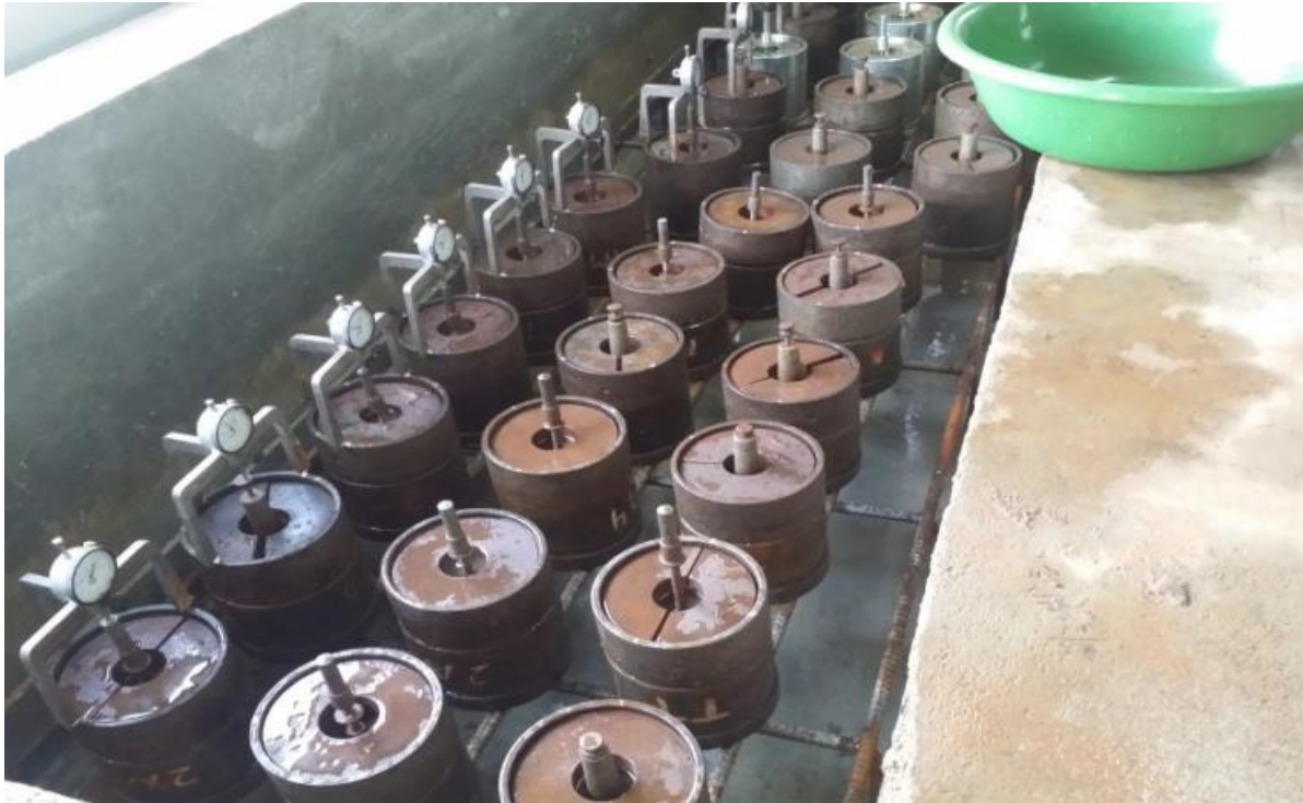
Figure 9: penetration of the sample for the CBR test.
